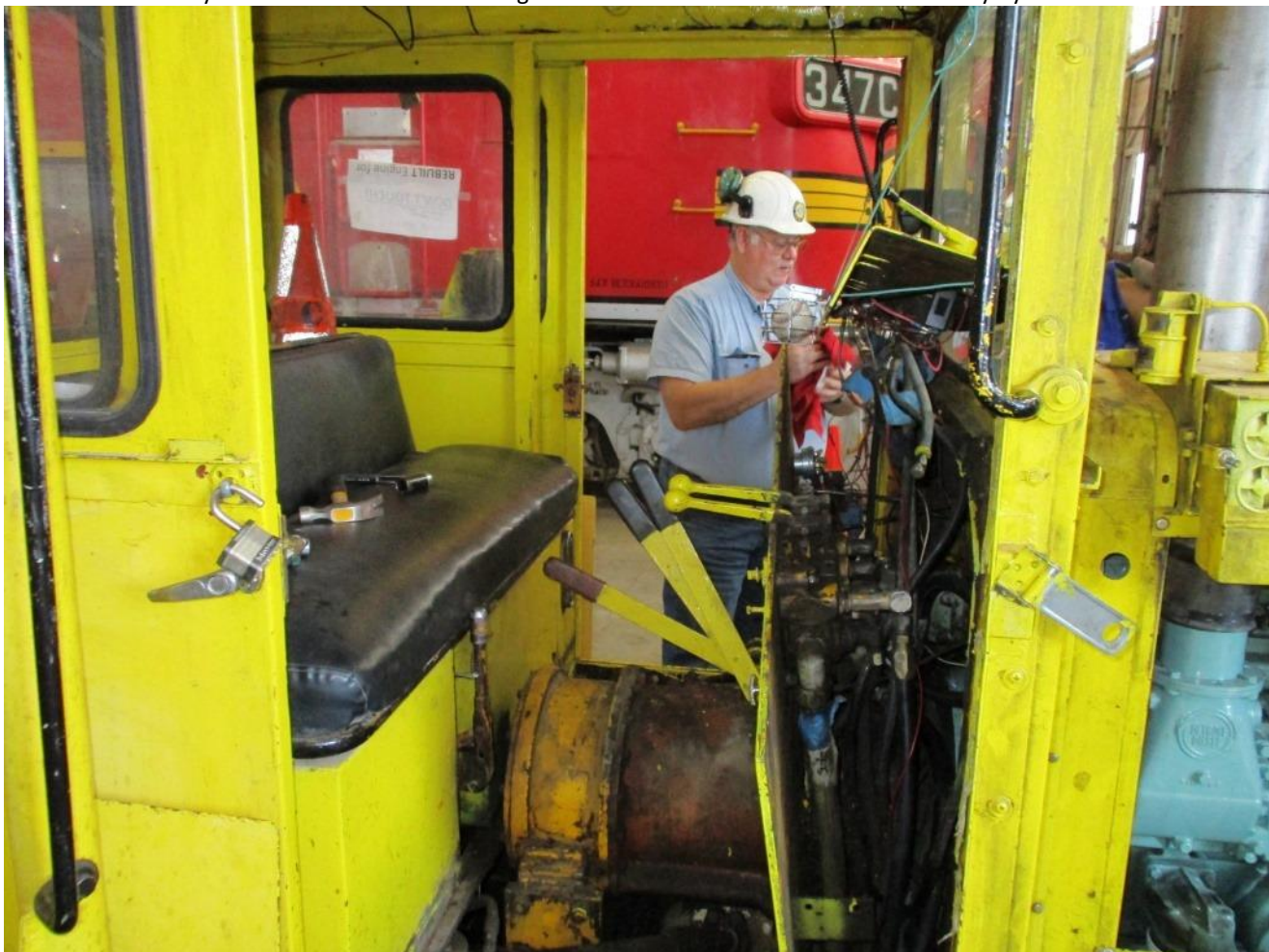
Whit the hose replaced, Chris C. cleans off the ignition switch
