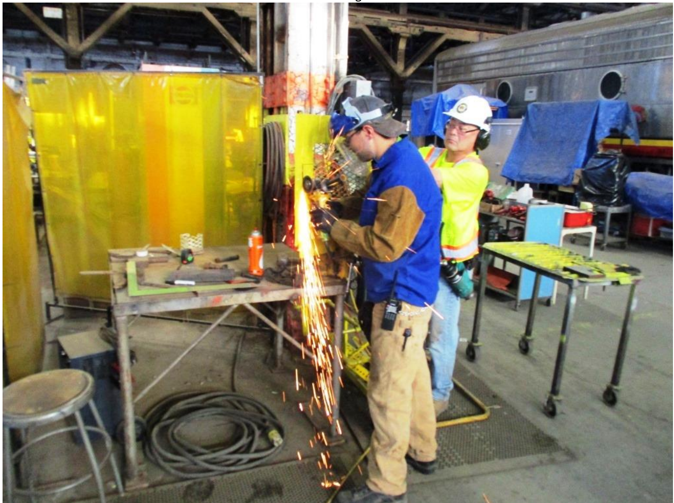
Kyle cuts the section of the engine shield being modified to fit new engine components
